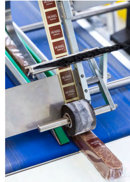
Field: Confectionary Application: Labelling chocolate bars
